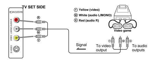
The figure below shows how to connect the SVHS input to video equipment.
